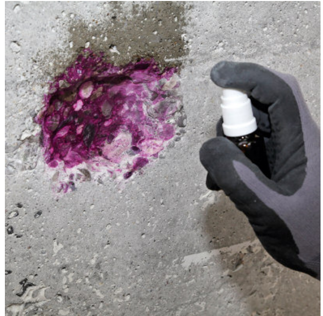
Here, the concrete provides adequate protection. The violet color indicates that the concrete is sufficiently alkaline.
