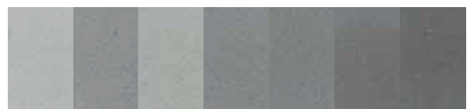
Differences in the color of exposed concrete caused by different types of formwork
